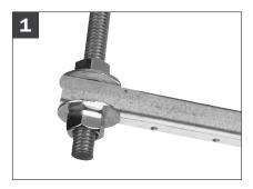
Locate holes on bracket and secure bracket to %" threaded rod using washers and %" nuts. If desired, hardware can be installed both above and below bracket. Install double nut if specified.
