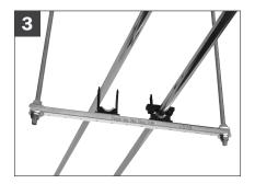
Position tube or conduit into base of TouchDown  $^{\text{TM}}$  clamp.
