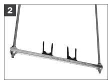
Slide  $TouchDown^{TM}$  clamps to desired location within the bracket.
