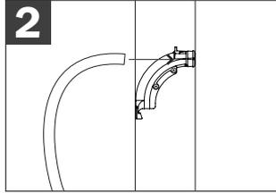
Insert end of tube into top 'nose' of plastic bend support.
