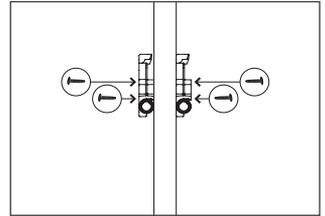
Two plastic elbows may be installed to straddle a stud for hot and cold supply.
