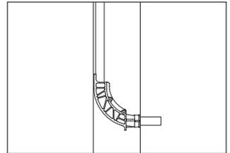
Plastic elbow may be installed on either side of stud, with flexible supply tube from above or below.
