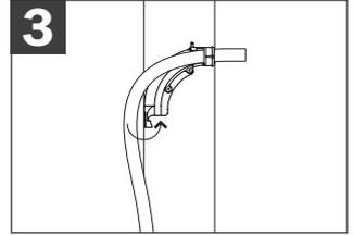
Holding opposite end of tube, guide tube through radius and around small hook on 'tail' end of the bend support.
