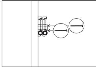
Using longer screws, two plastic elbows may be stacked against one side of the stud.
