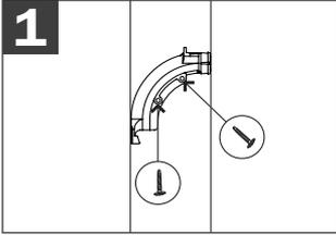
Using nails or screws, install plastic elbow directly to stud.
