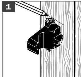
Hold Block 'A' up to vertical stud and mark position of block so that pipe is centered to stud's width.
