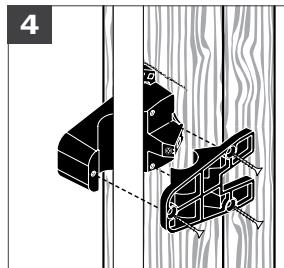
Gradually tighten each screw to secure blocks together starting at the front (nose).
