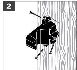
Attach Block 'A' to stud using each of the three pan-head drill-tip screws provided.
