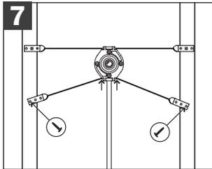
7 Secure ends of bottom bracket to studs.
