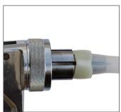
Failure to rotate tool inside tubing may cause unequal expansion. Remove any rings with unequal expansion.
