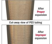
No rotation between expansions, or defective expansion head leaving a groove as a potential leak path.
