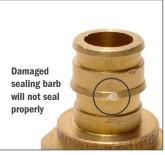
Damaged, cut or grooved barb on fitting.
