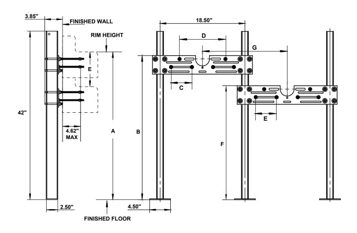
All feet to be secured to floor with 1/2" (min.) bolt and anchors - supplied by others
