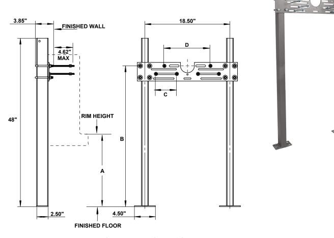
All feet to be secured to floor with 1/2" (min.) bolt and anchors - supplied by others
