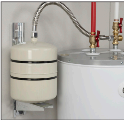
Attach the mounting column of the 2-pc. model using two or more screws (drive screws into studs) to support tank on an adjacent wall
