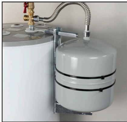
Hook the suspension beam of the 3-pc. model to the water heater nipple to support tanks vertically against the side wall of the heater tank. (Use extension piece for larger heaters)
