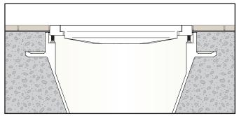
Install the adjustable frame and level with the new/added flooring. The separate frame allows the grate to be removed and replaced as needed.
