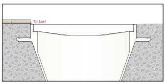
Even when fixture is installed flush/level with slab, adding tile or other flooring later can leave the grate too low, creating a trip hazard.
