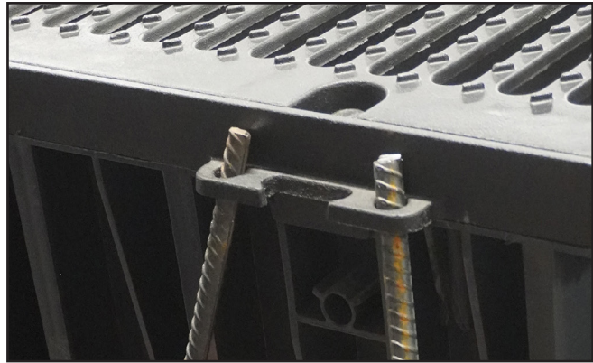
Grate frames include side anchor tabs. Tabs lock frames into the surrounding slab and work with 3/8" rebar to prevent movement before and during the slab pour.
