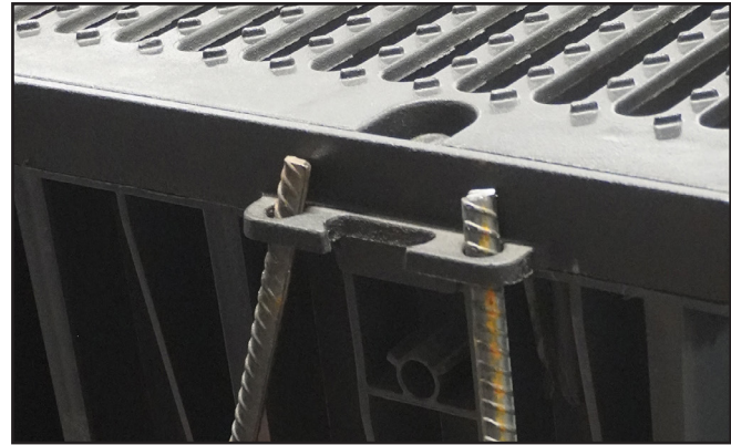
Grate frames include side anchor tabs. Tabs lock frames into the surrounding slab and work with 3/8" rebar to prevent movement before and during the slab pour.
