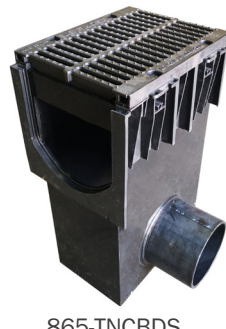
Grate frames include side anchor tabs. Tabs lock frames into the surrounding slab and work with 3/8" rebar to prevent movement before and during the slab pour.
